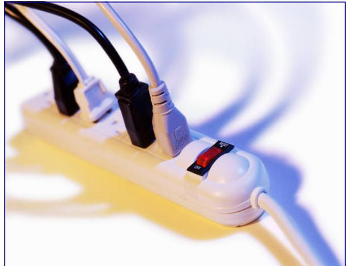
**Surge protectors are an inexpensive device used to protect electronic equipment from power surges. Prior to purchasing a surge protection device, make sure it states that it provides surge protection.**
